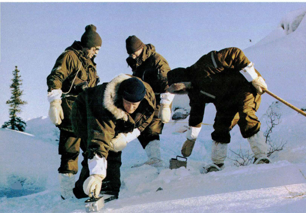
Above. A CF/scientific search team uses radiation meters to locate a small piece of radioactive debris. (EG&G photo 1571-24). Below. A scientist approaches debris found on Great Slave Lake. (EG&G photo 1501-16).
