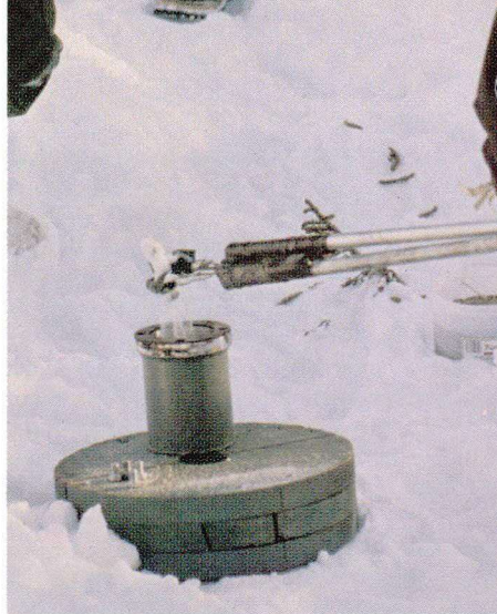
Far left. The pieces of the puzzle start to come together. (EG&G photo 1507-6). Using long tongs, a scientist places small pieces of radioactive debris in a lead container. (EG&G photo 1591-3).
