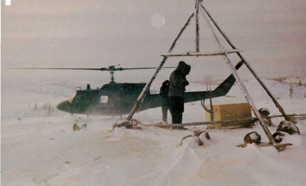
Above. A Twin Huey waits while a scientist prepares to change the batteries on a microwave ranging system beacon. In the extreme cold, the batteries had to be changed every 48 hours. (EG&G photo 1566-19).
