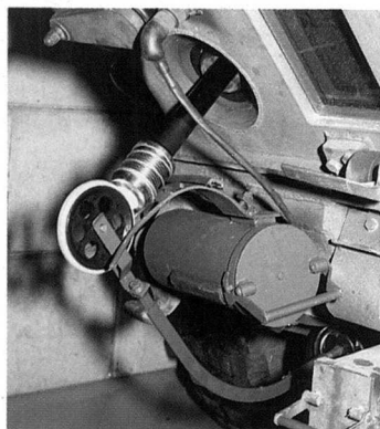
Ground probe and storage for spare detector wheels
