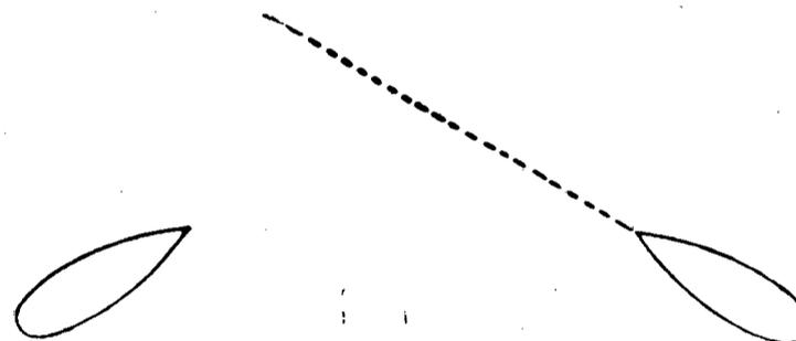
In this situation two steam vessels are approaching each other at right angles or obliquely in such manner as to involve risk of collision, other than where one steam vessel is overtaking another.
