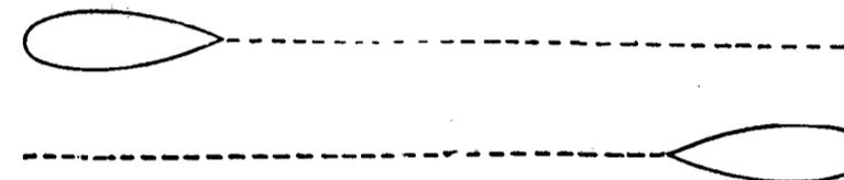
In this situation the green light only will be visible to each, the screens preventing the red light from being seen. They are therefore passing to starboard of each other, which is permissible in this situation, each pilot having previously signified his intention by two distinct blasts of the whistle.
