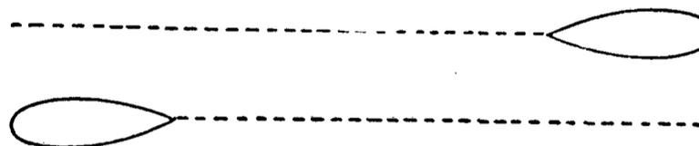
In this situation the red light only will be visible to each, the screens preventing the green lights from being seen. Both vessels are evidently passing to port of each other, which is permissible in this situation, each pilot having previously signified his intention by one distinct blast of the whistle.
